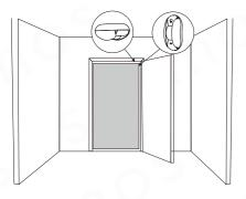
**Note:** make sure the detection direction faces towards the interior, no matter it is installed on wall or at ceiling. Adjust the bracket angle to optimize the detecting effect.
