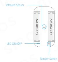
Infrared sensor: Detecting human body's infrared spectrum. Don't touch the surface by hand and keep it clean.
